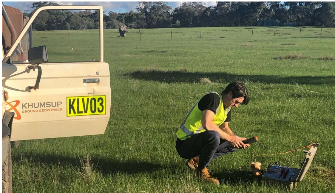
Figure 2 Dipole/Dipole Induced Polarisation survey at Darlington Prospect.
