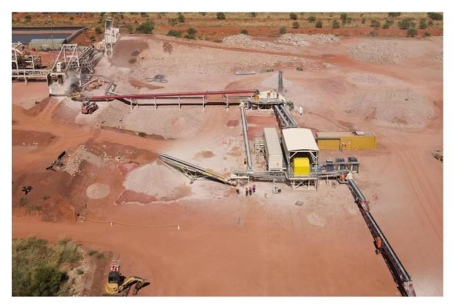
Figure 1: Operational ore sorter system
