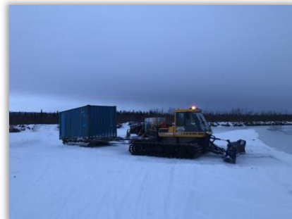
Photo 2-3: Typical snow road freight haul operations in same area as Estelle Gold Project route. Winter road operations bring significant saving from freight costs and allow resource development work to continue unabated year round. Work on road maintenance and freight continues 24/7 during winter months until the job is complete.
