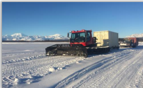
Photo 2-3: Typical snow road freight haul operations in same area as Estelle Gold Project route. Winter road operations bring significant saving from freight costs and allow resource development work to continue unabated year round. Work on road maintenance and freight continues 24/7 during winter months until the job is complete.
