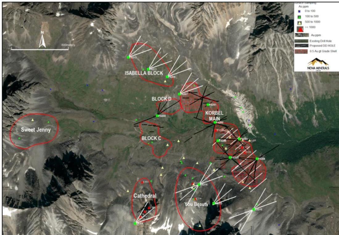
**Figure 4. Korbels Main Drill Hole Layout**
