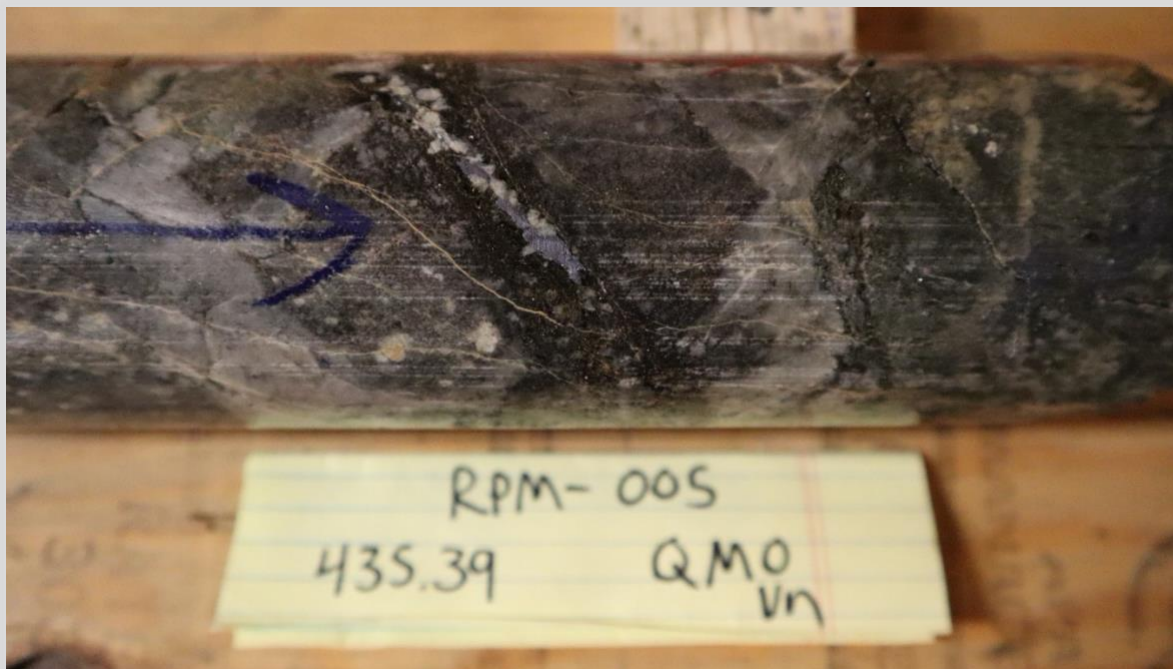
Figure 4b. RPM-005 selected core showing highly fractured intrusive host with Au bearing qtz-moly veining at 132.7 meters (435.39 feet) depth within sample interval returning 24.5 g/t Au .
