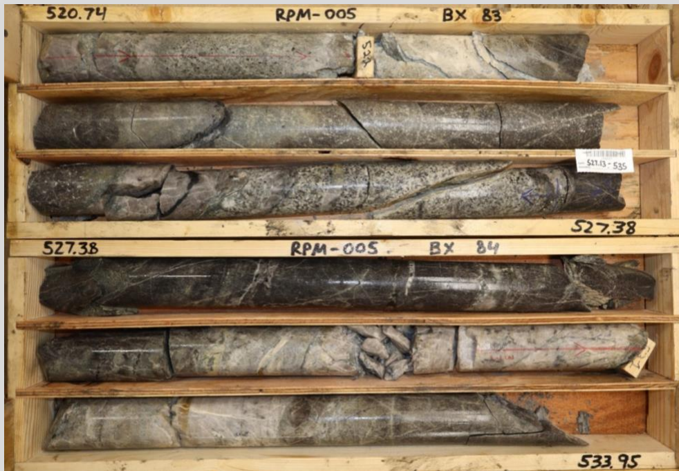
Figure 3b. RPM-005 drill core interval 159-163 meters (520.74-533.95 feet) depth returning 50.3 g/t Au . Typical mineralized structure and veining within intercalated hornfels (dark) and qtz-feldspar intrusive dyke (light) host rocks.
