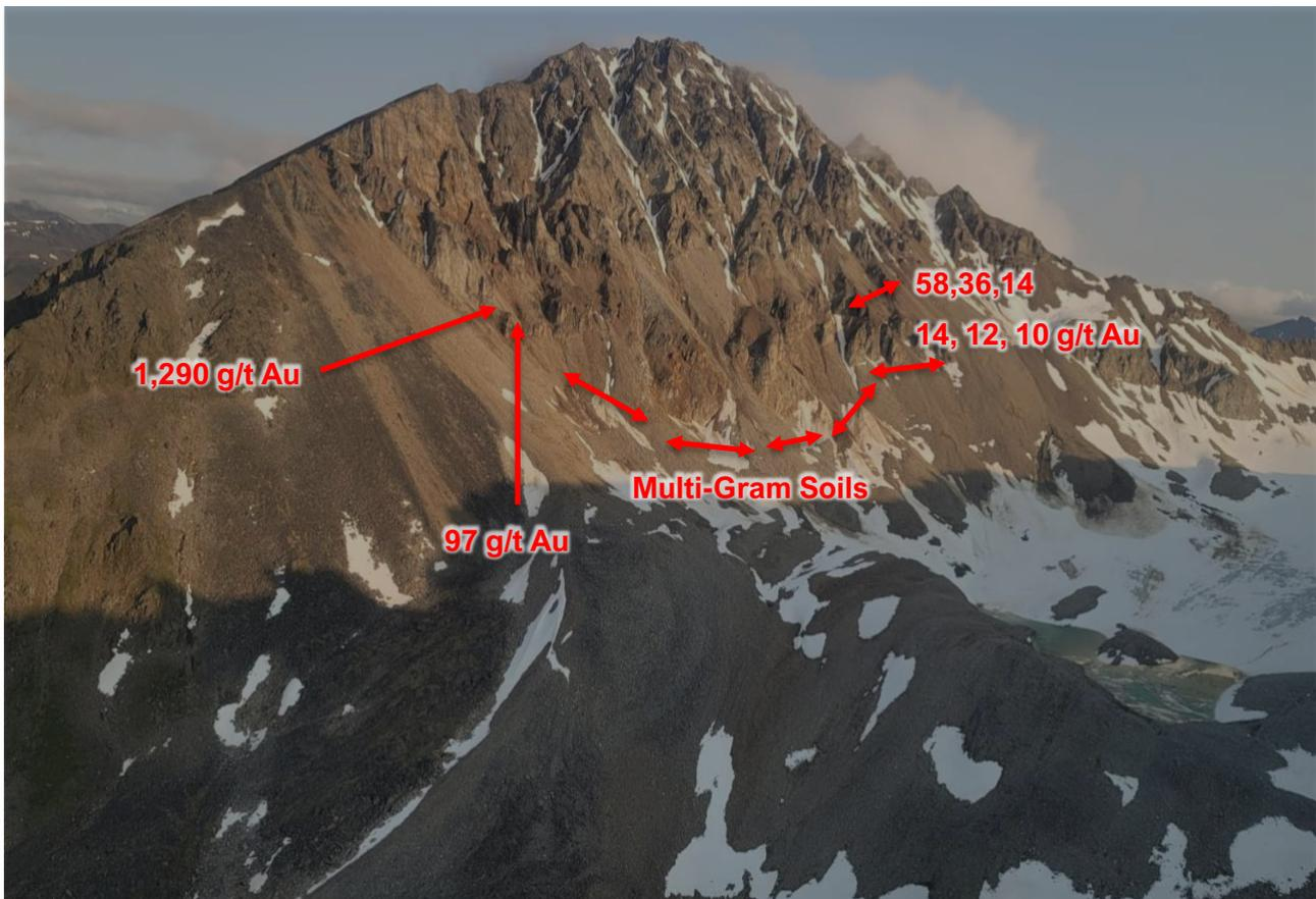
**Figure 4.** View of Shoeshine looking to the West, with high-grade surface samples
