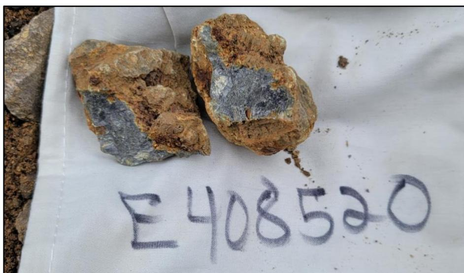
**Figure 2.** Sample E40820 – 1,290 g/t Au, 0.9% Sb, 591 g/t Ag, 1.0% Cu, 1,300.1 g/t AuEq talus sample collected in chute
