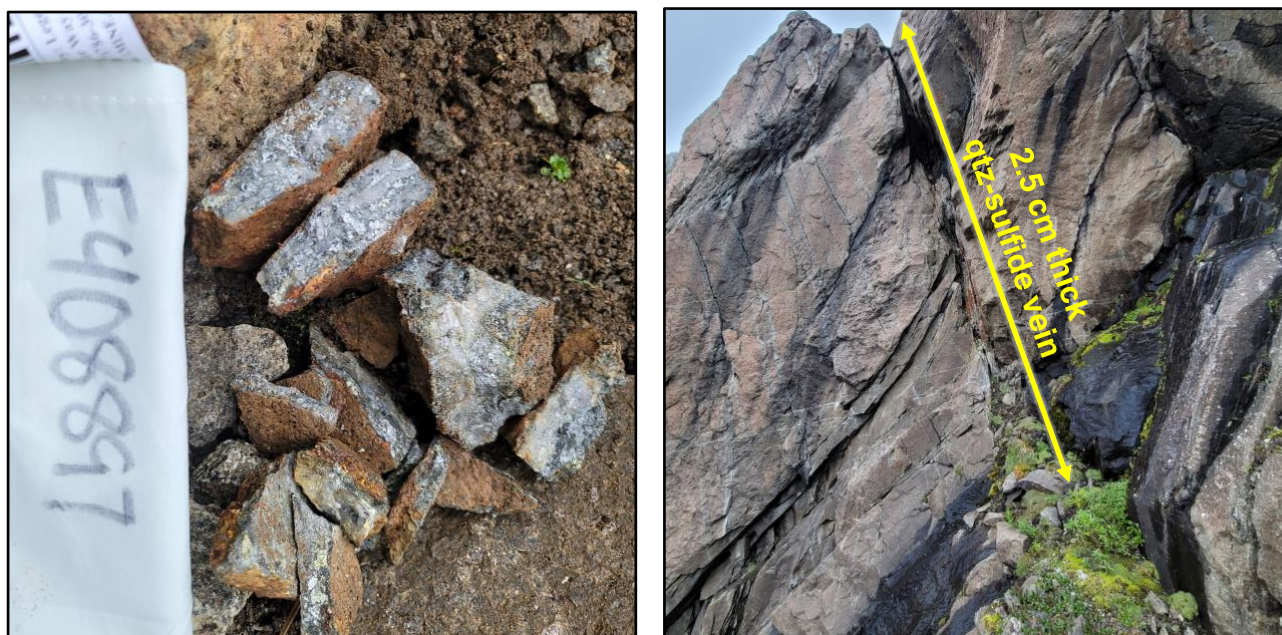
Figure 3. Vein-hosted mineralization; Sample 408894 – 20.9 g/t Au, 55ppm Ag, 1.3% Cu, 600 ppm Sb, 23.0 g/t AuEq
