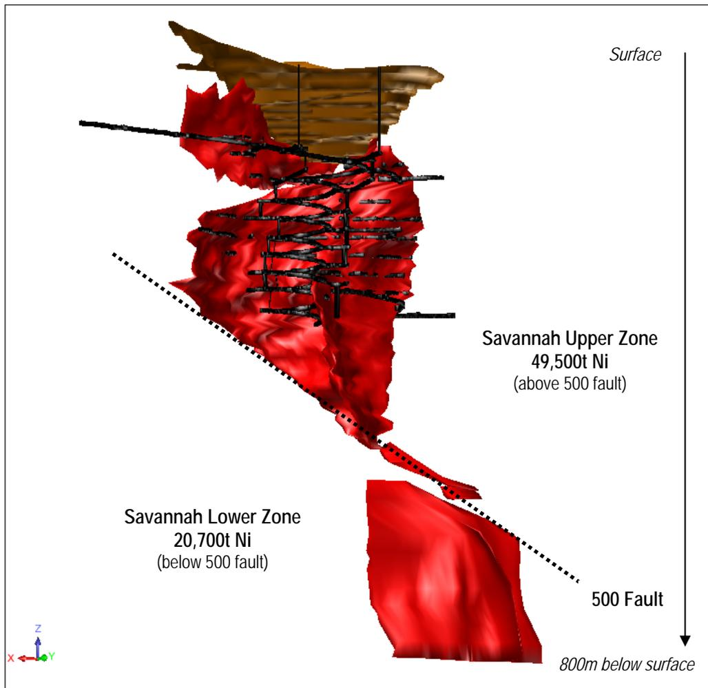
Figure 1: Three dimensional representation of the Savannah Mineral Resource
