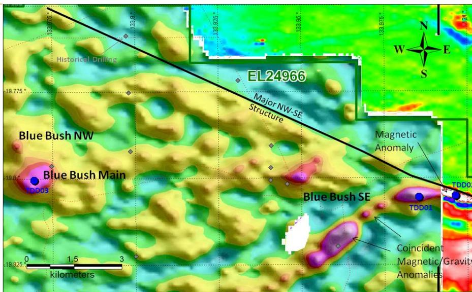
Figure 1 - Drill hole location map over residual gravity image (left of image) and TMI 1VD magnetic image (right of image).
