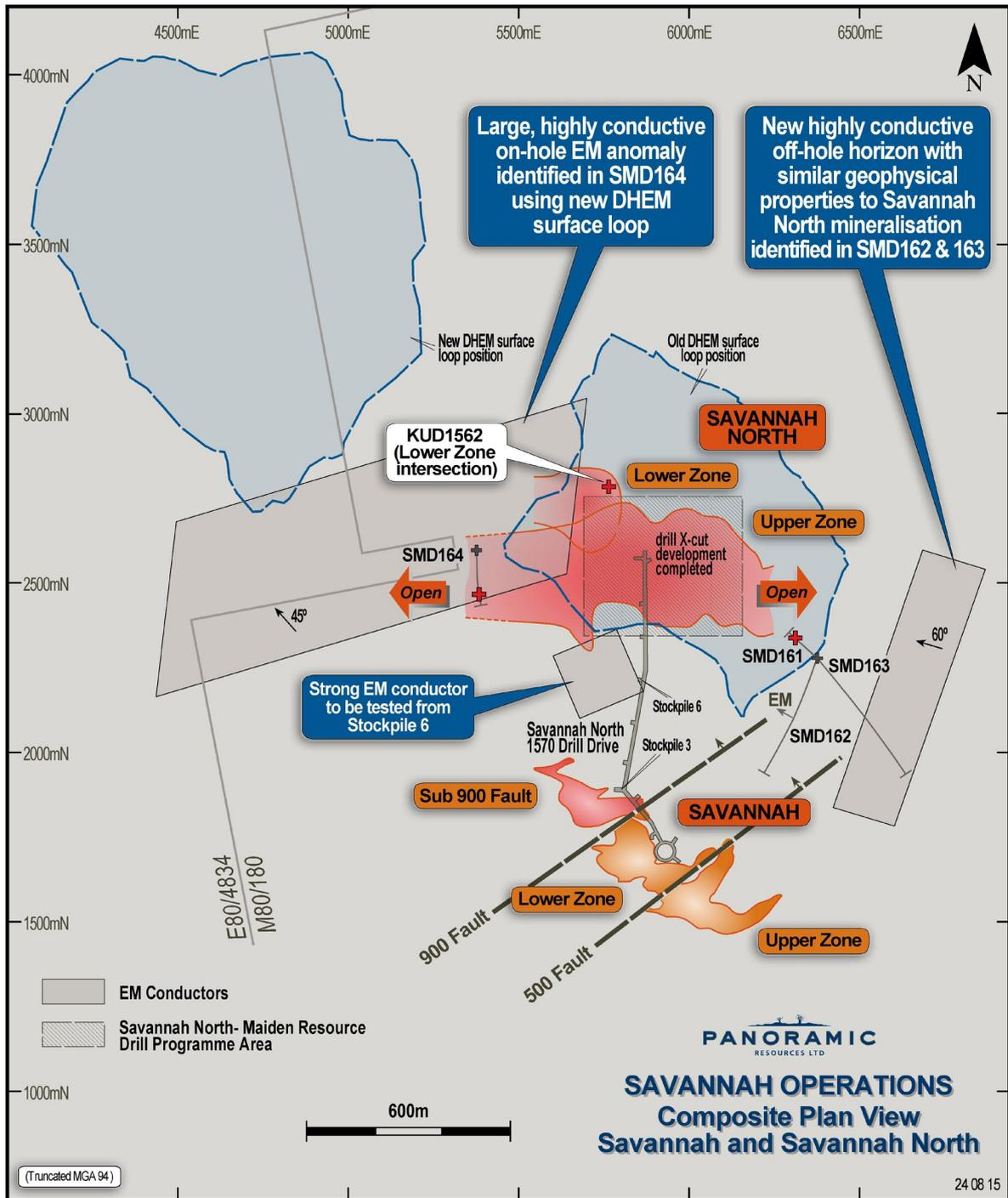
**Figure 3-3: Composite plan view of the Savannah and Savannah North deposits**
