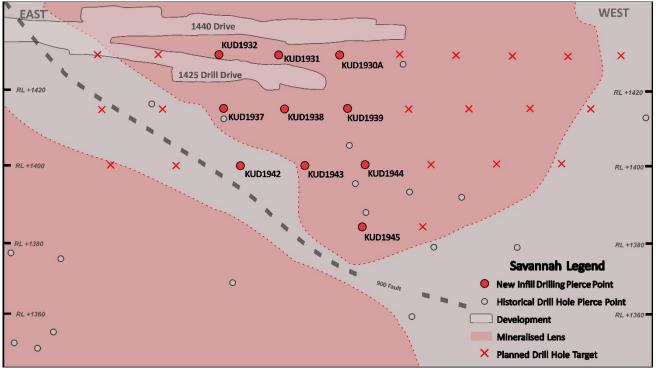
Figure 3: Long-section of the Resource definition drilling at Savannah and historic Resource definition drilling intercepts with development drives and proposed drilling
