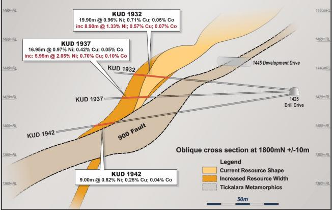
Figure 2: Oblique cross section at 1800mN +-10m showing drill holes KUD1932, 1937 and 1942, current Resource shape and proposed mineralisation model
