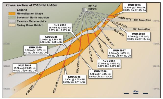
Figure 2: Savannah North cross section 2510mN showing recent drill intercepts below the 1321 level
