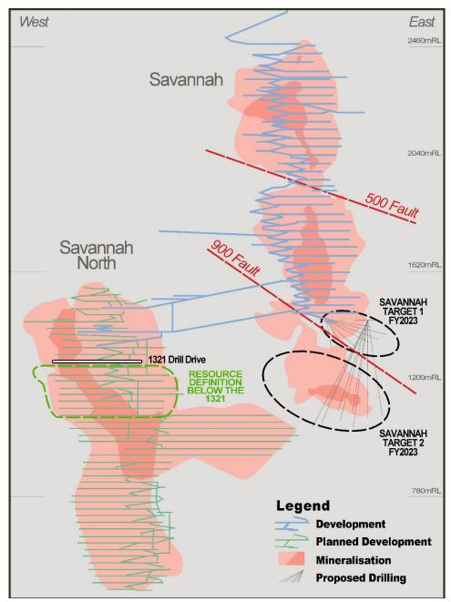
Figure 1: Schematic of target drilling area below the 1321 at Savannah North
