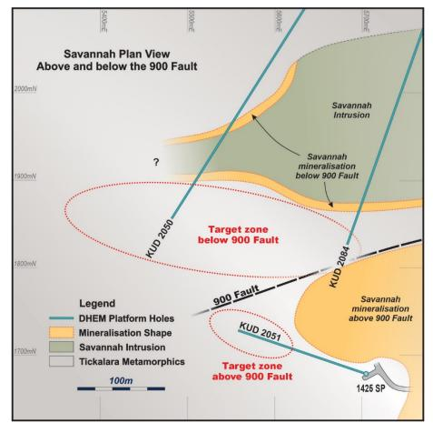
Figure 1: Plan view of the DHEM platform holes targeting Savannah above and below the 900 Fault
