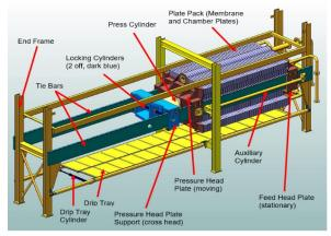
Figure 1. Filter Press and location of Pressure Plate Support (Cross Head) which failed (Blue)
