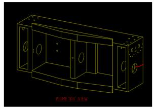
Figure 2. Isometric view of pressure end with original crack shown in red
