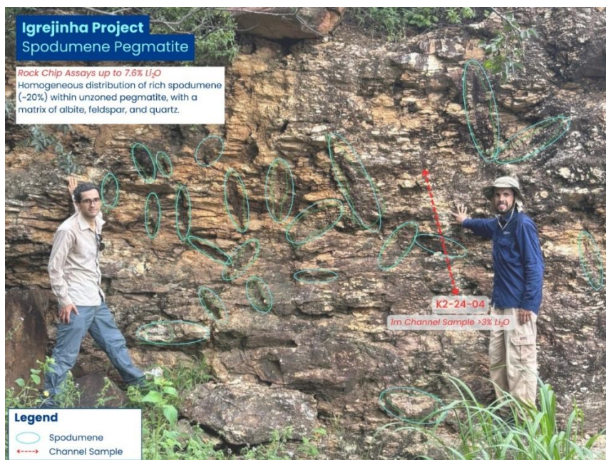
Figure 6– Outcropping spodumene-bearing pegmatite at Morro Grande (within the Igrejinha License 830851/2010), which contains individual spodumene crystals up to 50cm in size. Channel sample K2–24–04 also shown, which assayed at 3.26% \text{Li}_2\text{O} . 11
