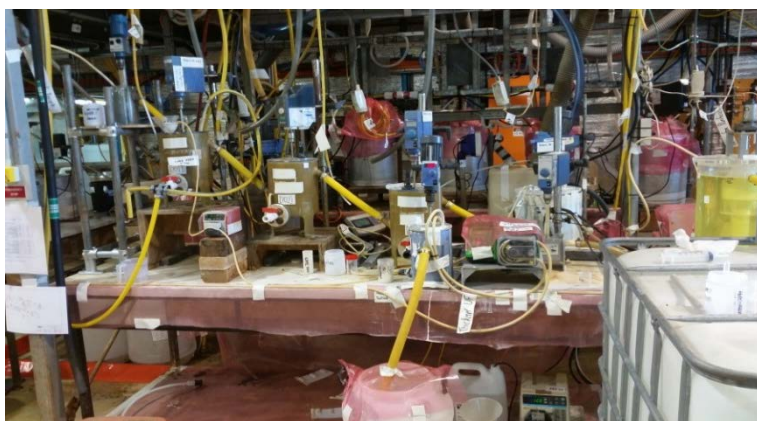
Figure 6: Effluent Treatment Circuit
