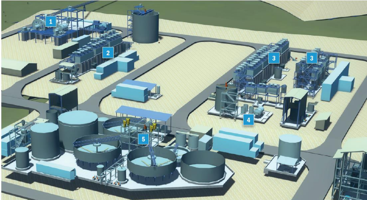
Figure 3: Ngualla plant 3D layout comprising of (1.) SAG & ball milling, (2.) Barite pre-float circuit, (3.) Rare earth flotation circuits, (4.) Re grind circuit and (5.) Concentrate & tailings de-watering
