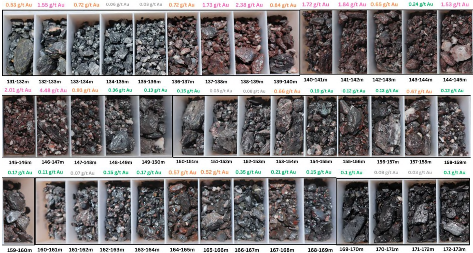
Figure 11. RC drill chips from BSRC007 for intercept 42m @ 0.66g/t from 131m (incl. 17m @ 1.3g/t Au from 131m) from Garibaldi showing mineralised zone defined by quartz veining & pyrite in siltstone-shale unit with hematite staining and chlorite alteration.
