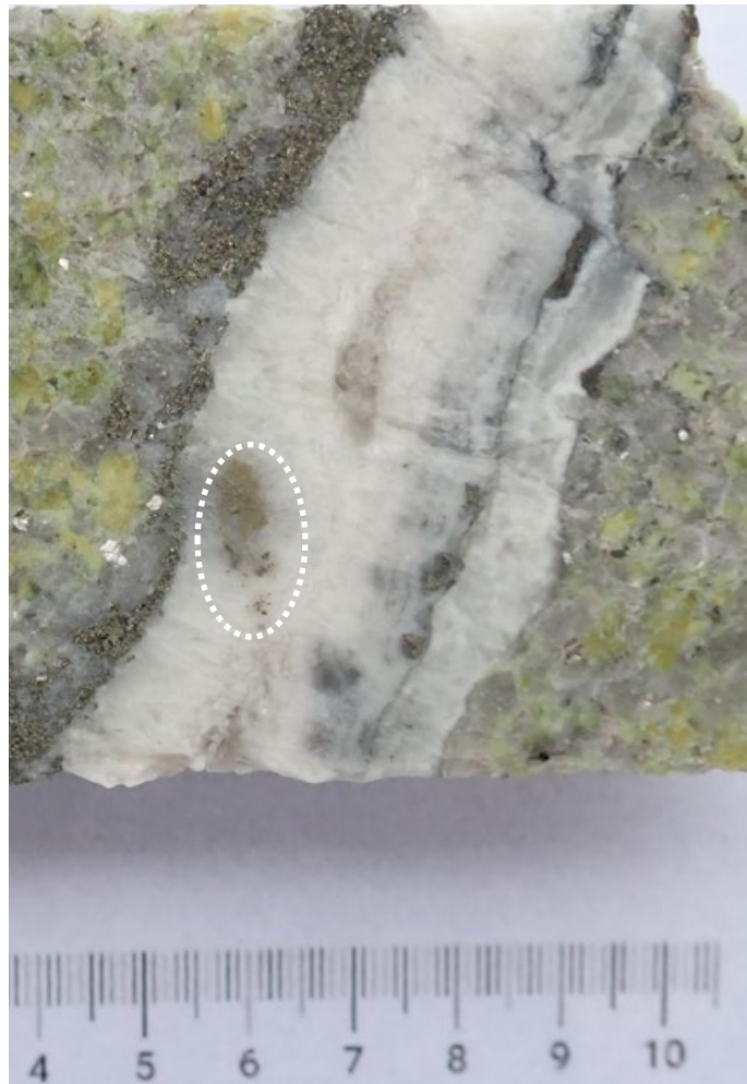
Figure 3: Banded epithermal quartz with fine-grained internal sulphide banding and coarse pyrite on vein margin at 88.9m. Visible gold encapsulated within the vein, assays pending.
