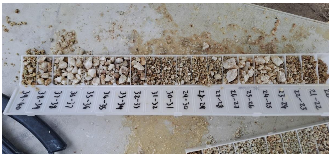
Figure 5: Reverse Circulation drilling on the Shadows Prospect at Alice River Gold Project. Note the quartz vein intersections from 23m to 27m, and 32m to 40m in samples from drillhole SHDH012.
