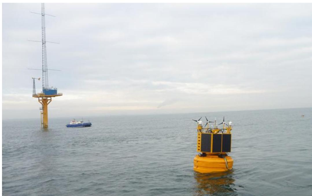
Figure 3 Tradition met mast structure compared to a LiDAR system
