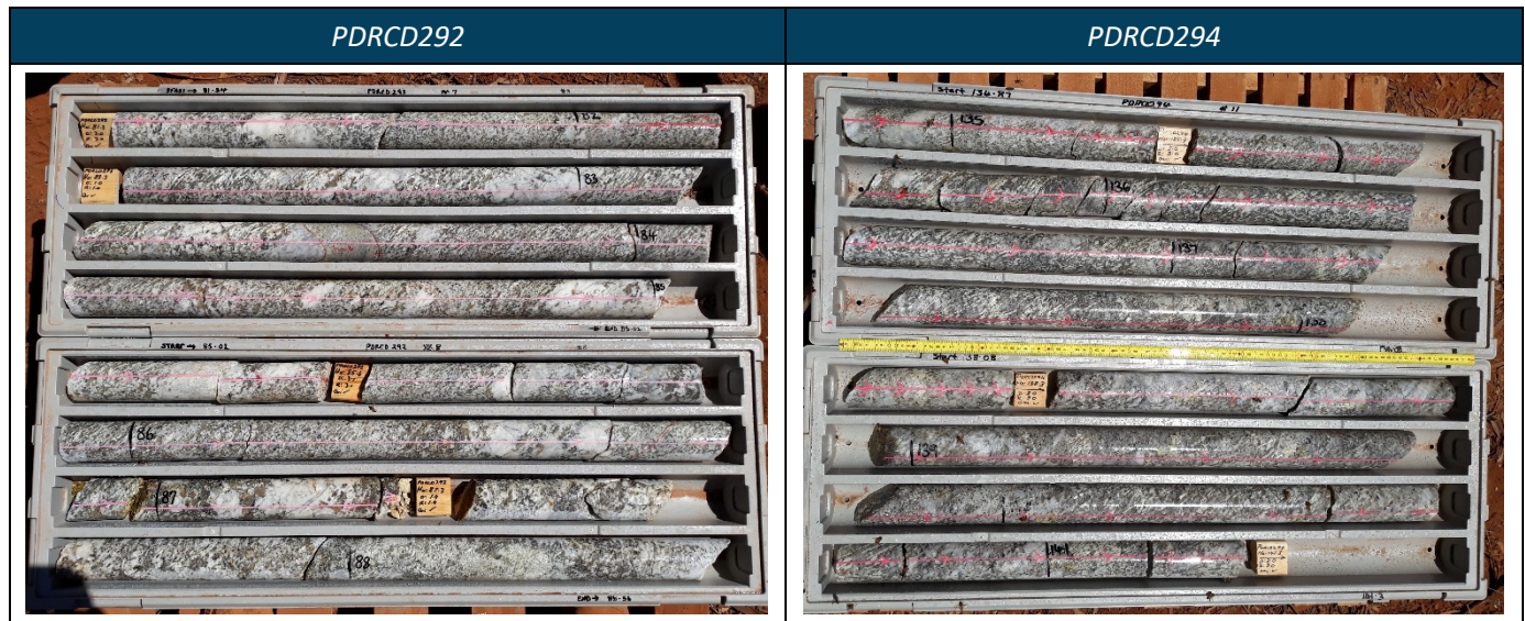
Figure 3: Pioneer's geologists have identified spodumene-pegmatite in drill core from holes PDRCD292 and PDRCD294 drilled during the current programme.
