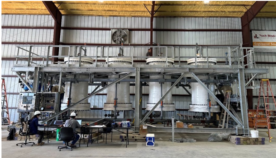
Figure 2: Engineers Assessing Prairie Lithium's four column Commercial Scale DLE Unit during FAT
