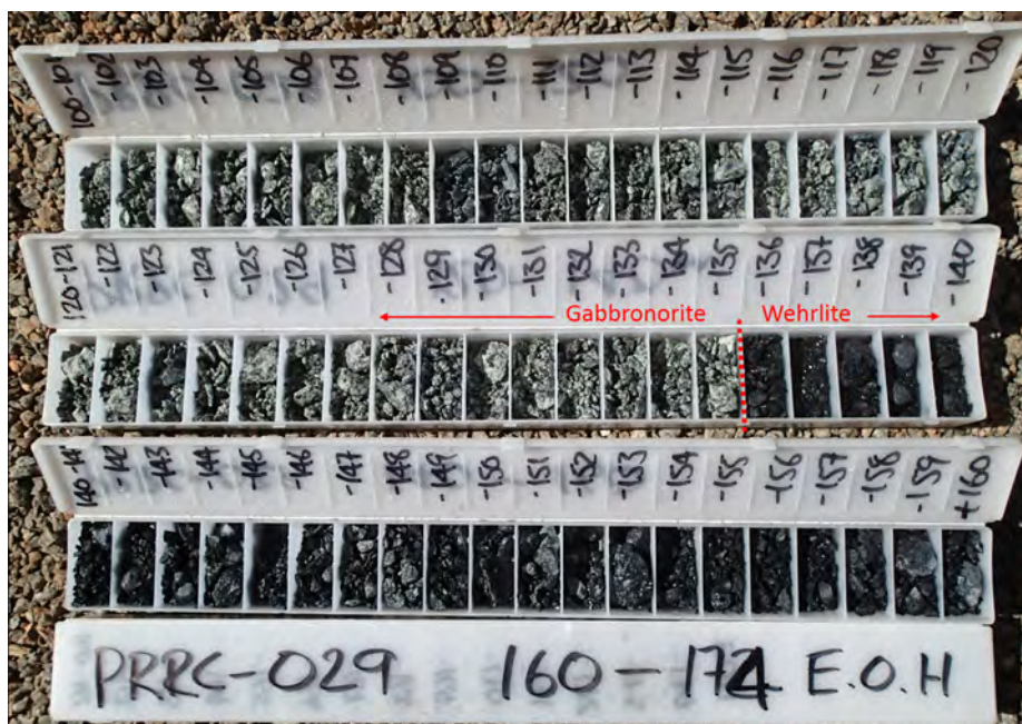
Figure 3 - Gabbronorite-wehrlite contact in RC hole PRRC029
