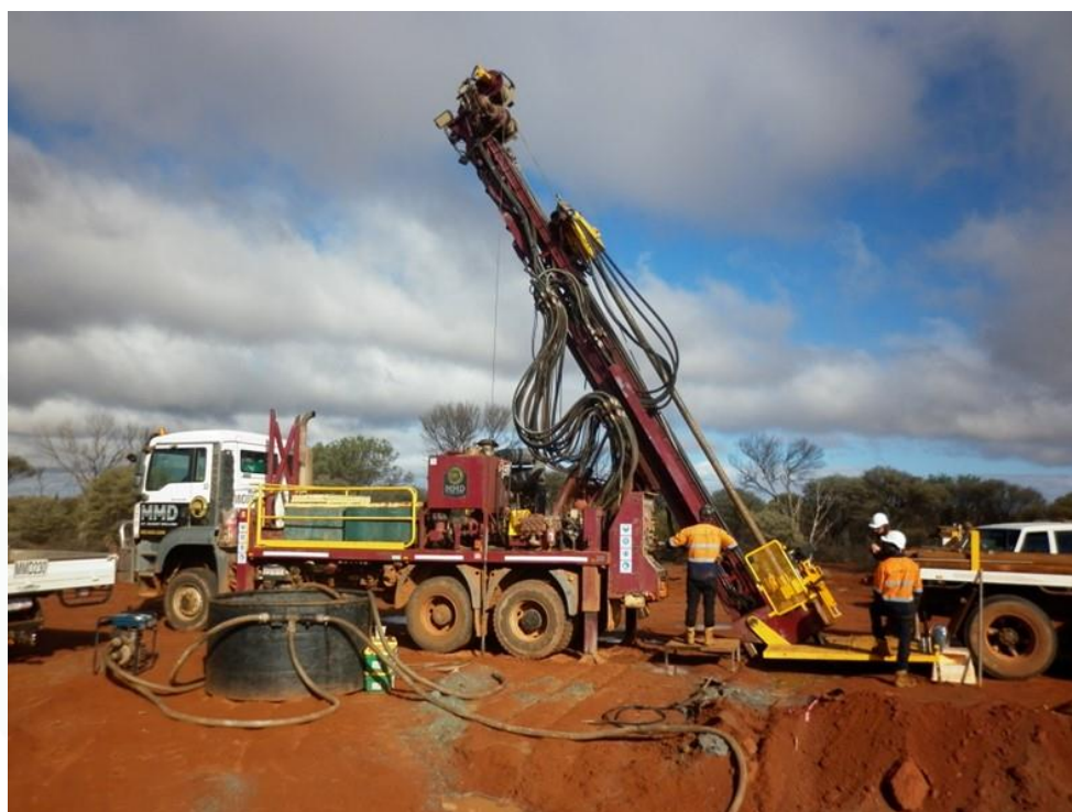
Figure 12 – Stage 10 diamond core rig drilling core tails
