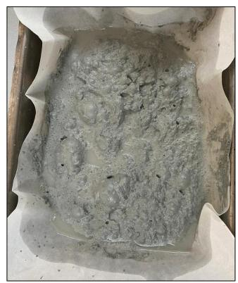
Rougher concentrate from laboratory flotation test
