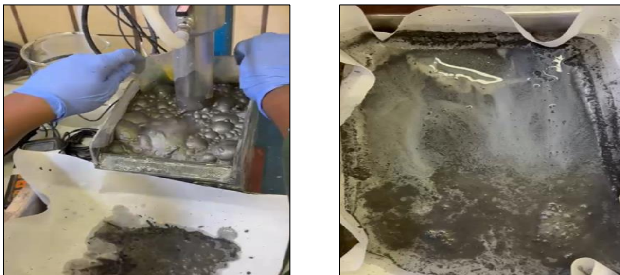
Figure 11: Copper Flotation Test (left) and Copper Rougher Concentrate (right)
