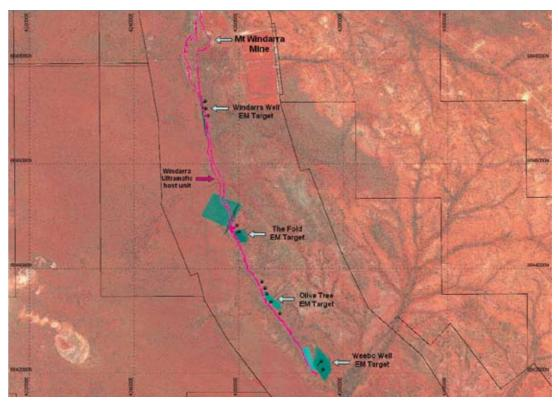
Aerial photo of the Windarra Nickel Project showing EM plates with planned drill hole positions at prospective targets.
