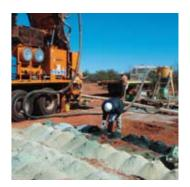
A geologist is seen here testing rock chips using a Niton XRF gun.
