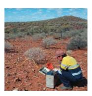
The discovery of 7 well defined lava channels led to the redeployment of Electromagnetic testing at Windarra. Rather than broad testing, the Company was able to focus on individual locations to prioritise the drill program.
