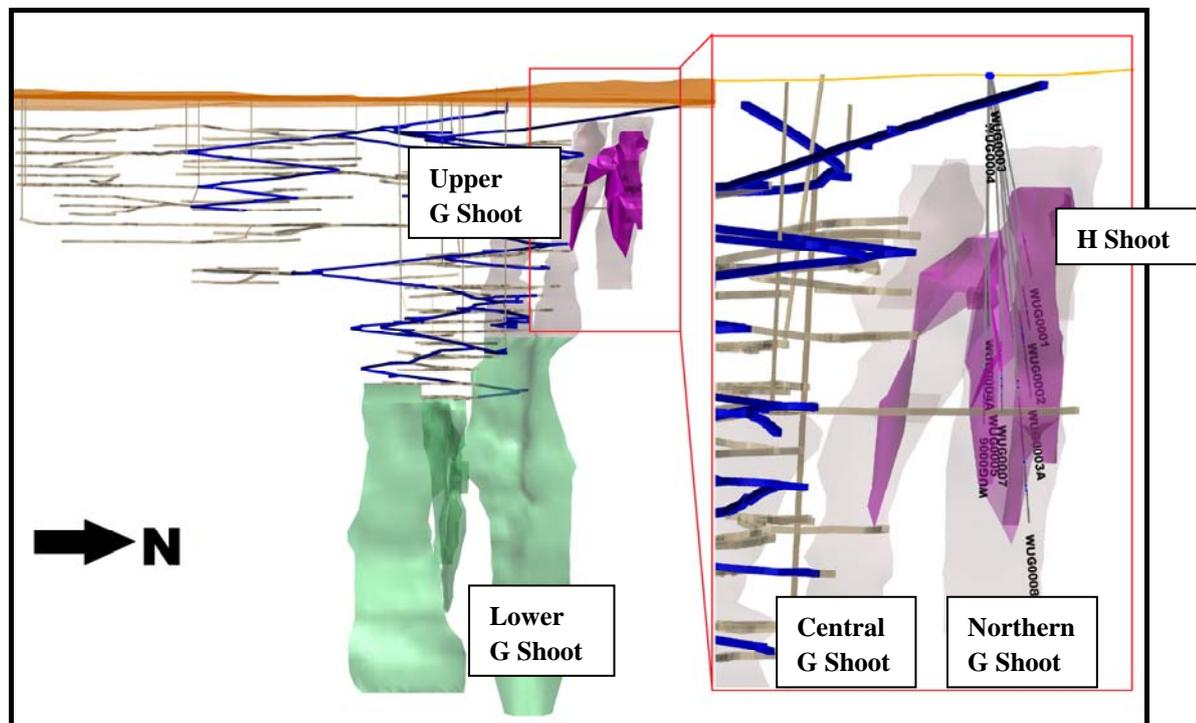
**Figure 1:** 3D model of the Windarra mine showing the defined ore shoots with respect to the mine decline (blue) and development (grey). The newly defined H Shoot is defined by the dark purple shape, with Upper G Shoot (light grey) and Lower G Shoot (green) shown relative to the H Shoot position. The positions of the reported drill intersection are shown on the expanded inset.
