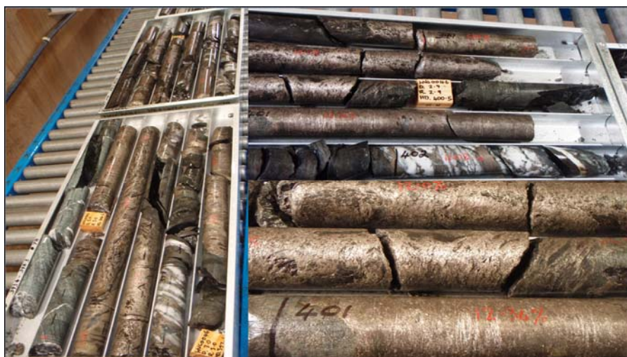
Figure 2: High grade massive sulphide intersected in D Shoot by WUG0046
