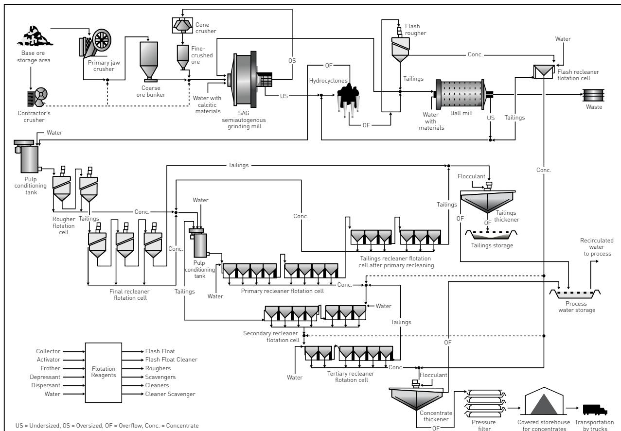
Figure 1: Black Swan overall process flow diagram
