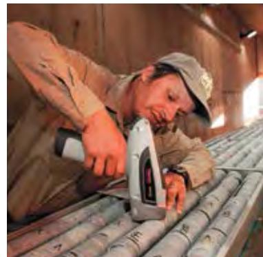
Innovation has saved us time and money. This portable XRF analyser is able to give us critical insights into rock mineralogy in real time rather than in weeks previously. We can now constantly adjust our drilling programmes using fast feedback even as a hole is being drilled.
