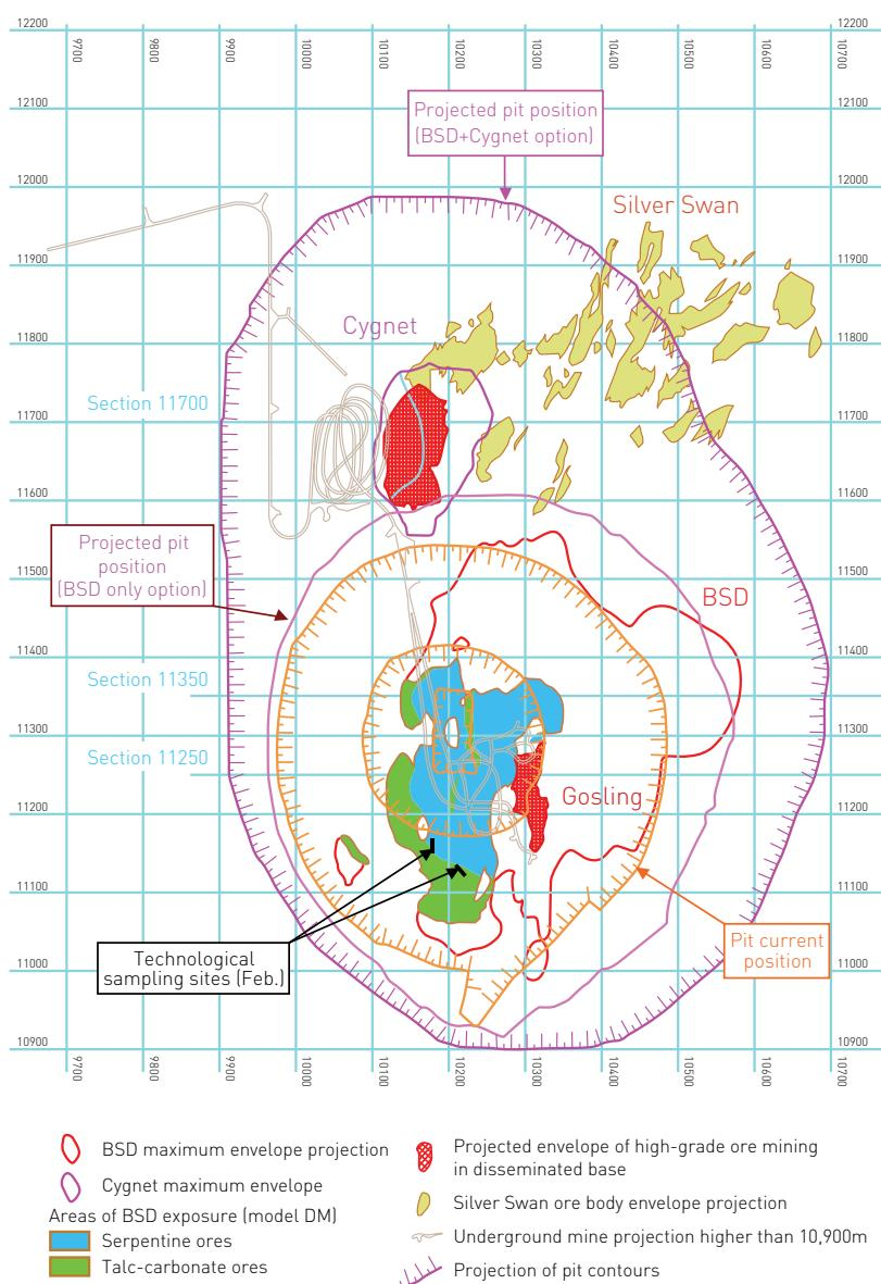
Figure 4: Black Swan Disseminated (BSD) and Cygnet mineralisation with existing mining infrastructure and pit shell options
