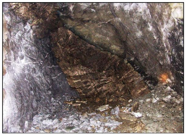
Figure 2: Goose 10170 level (now mined) showing high grade massive nickel sulphide (~13% Ni) in the ore drive.
