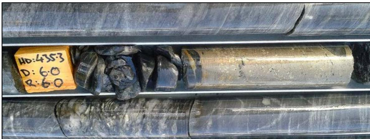
Figure 1: Narrow stringer of remobilised nickel sulphide grading 10.2% Ni in PLJD0001
