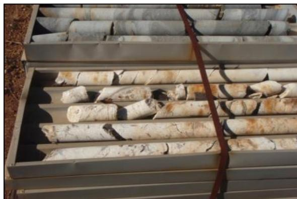
**Figure 5: The core yard holds many trays containing thick intersections of unsampled pegmatites (white rocks) as they have always been considered barren waste rock until the significance of these potential lithium-tantalum bearing pegmatites were recently recognised**
