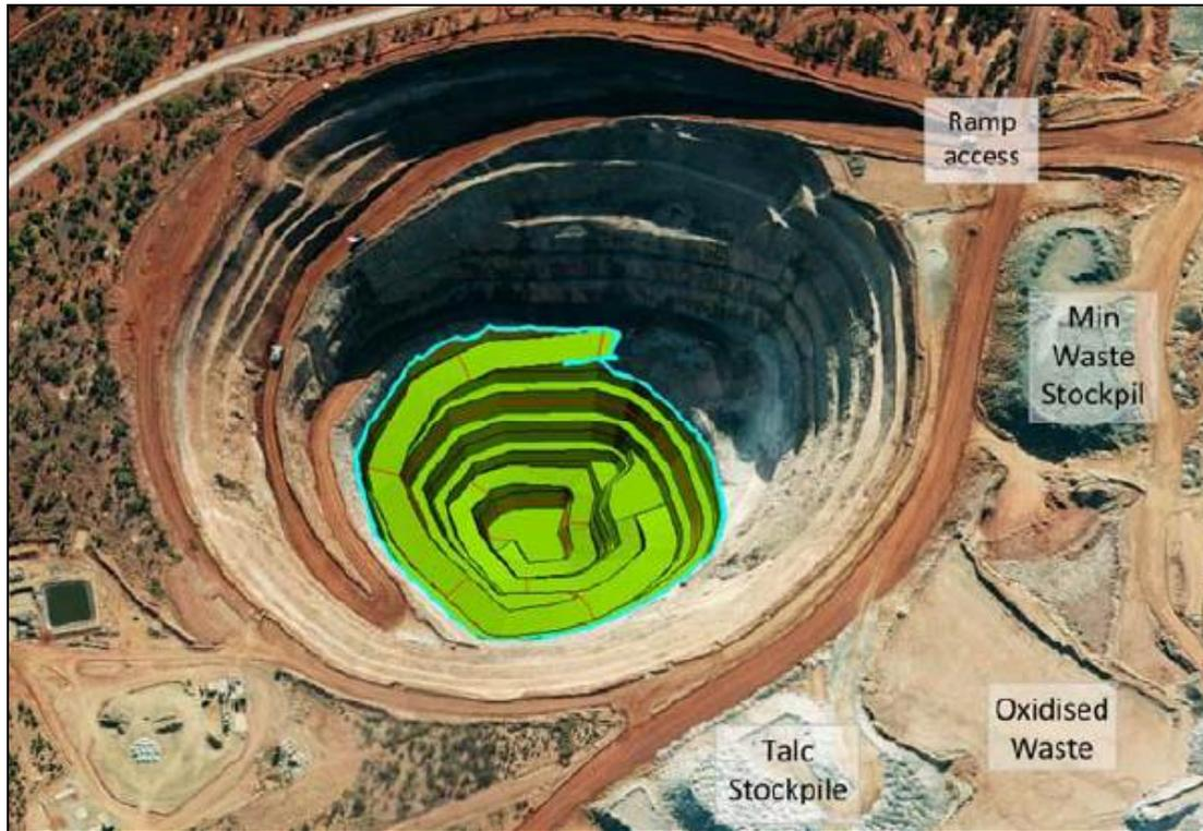
Figure 3: Black Swan open Pit (development at the bottom of existing pit)
