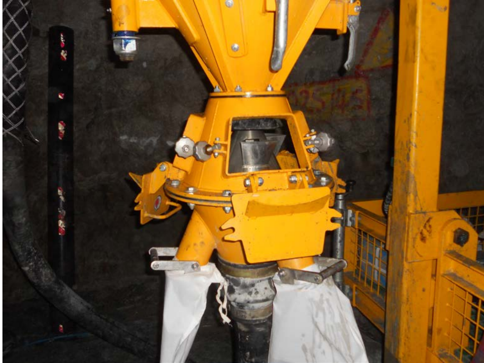
Figure 3- Purpose built underground RC rotary splitter
