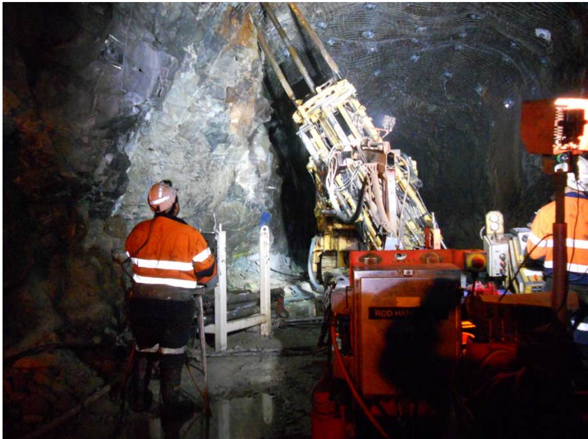
Figure 2- Underground RC drill rig in use
