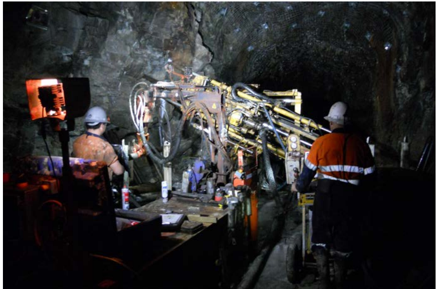
Underground RC drill rig at Black Swan
