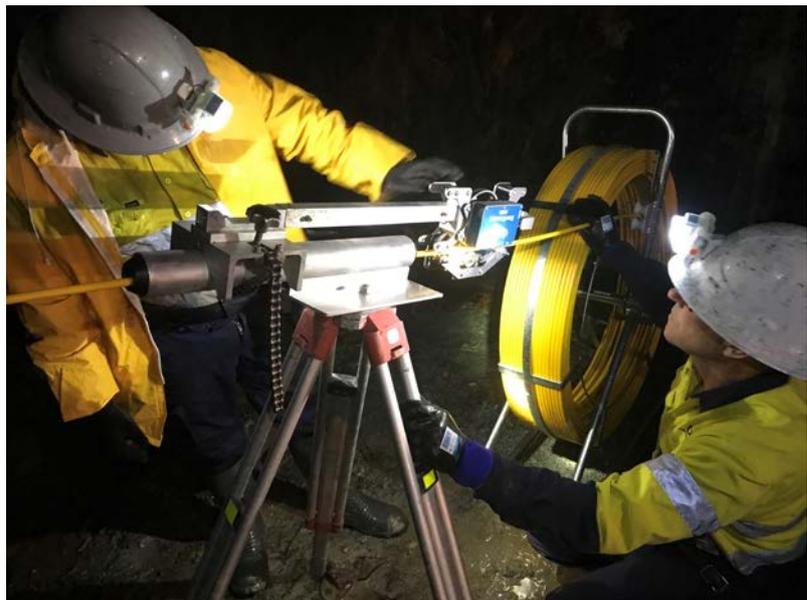
Figure 1: Full up-hole continuous gyro survey
