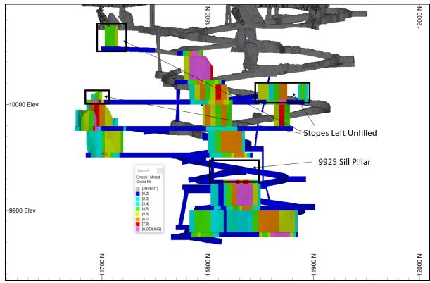
Figure 1 - Ore Reserve Estimate Mine Design (Long-Section Looking W)
