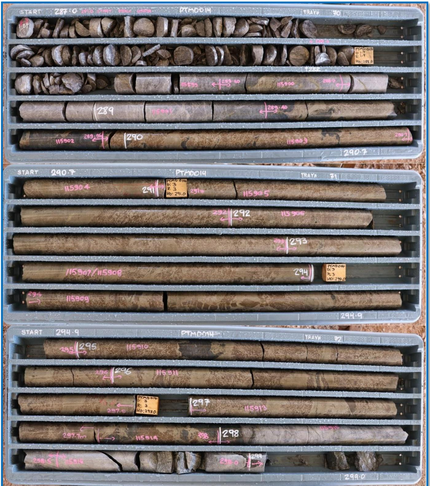
FIGURE 1: VISUAL MASSIVE SULPHIDES IN HOLE PTMD014 FROM 289.95M
