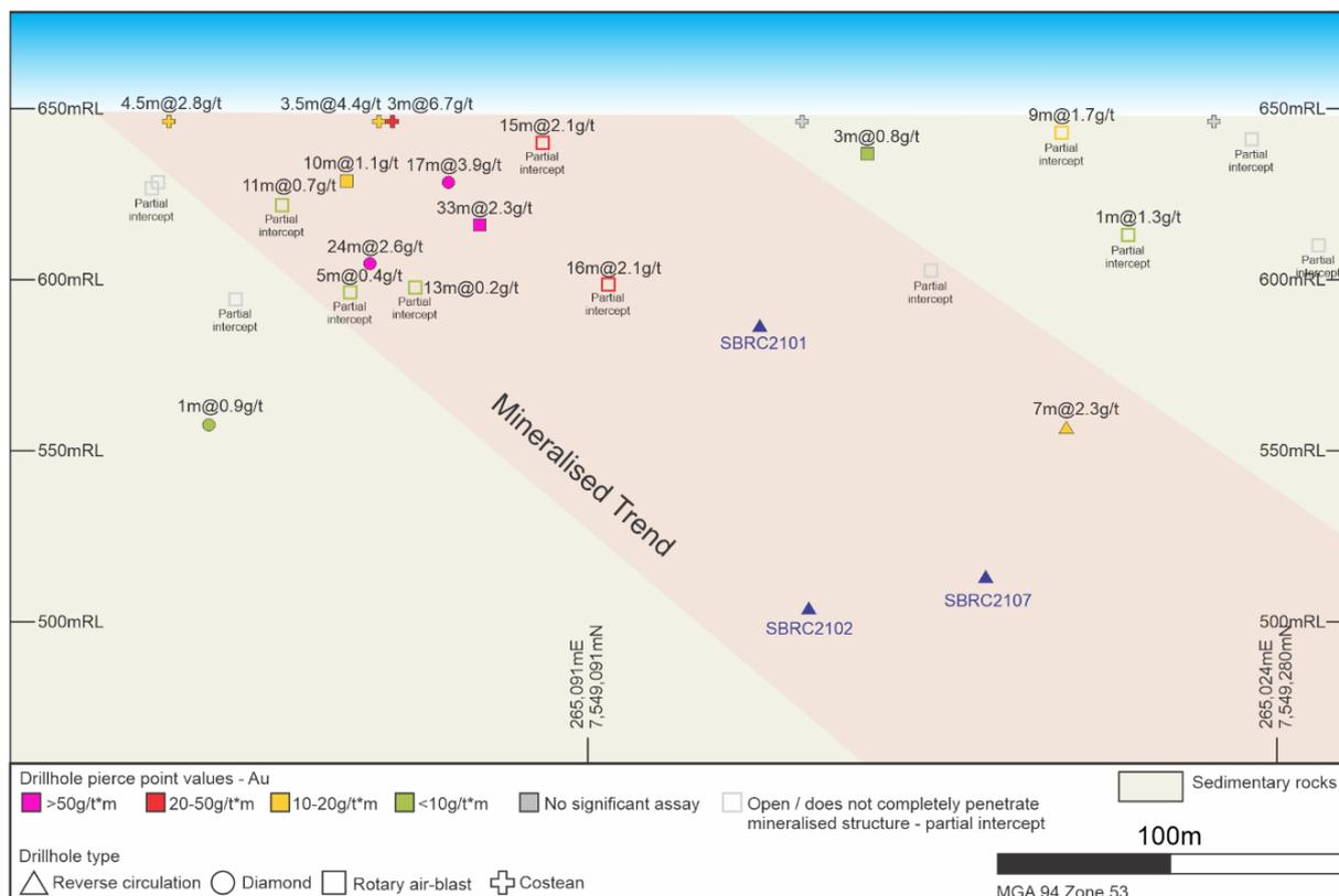
Figure 3 - Longitudinal Projection (Long section) showing the position of recently completed holes at Sabre. (Previous results ASX: 18 January 2010)
