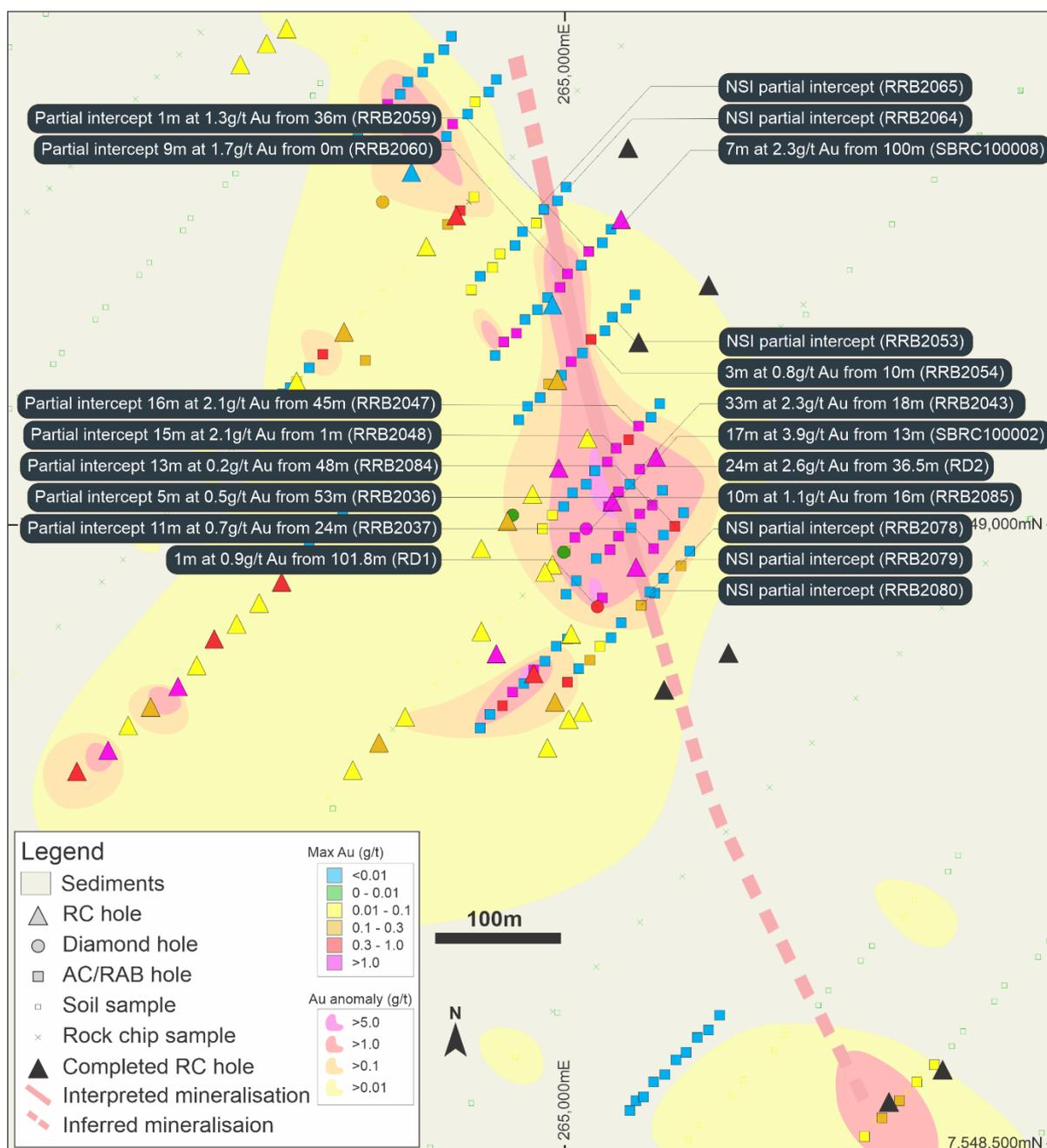
Figure 2 –Sabre Prospect gold anomalism (ASX: 18 January 2010) and RC drill holes completed in May 2021
