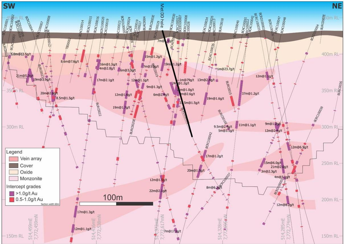
Figure 6 - Oblique section showing approximate position of the May 2021 metallurgical hole
