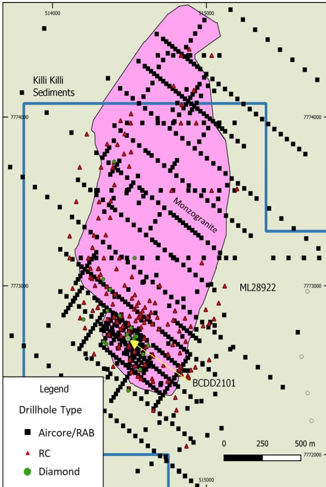
Figure 7 - Buccaneer Prospect showing existing drilling and the recently completed diamond hole BCDD2101
