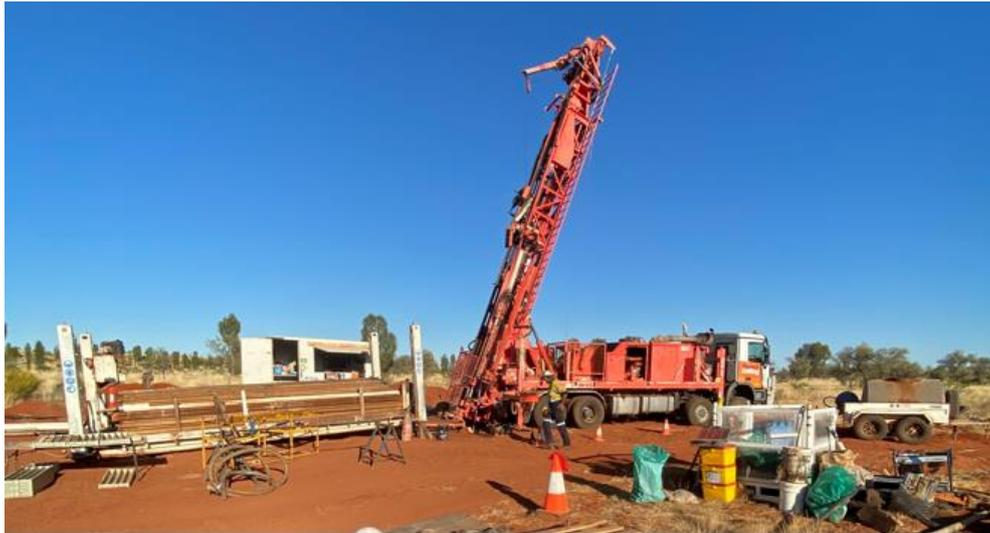
Figure 2 – Diamond drill rig at Phreaker prospect
