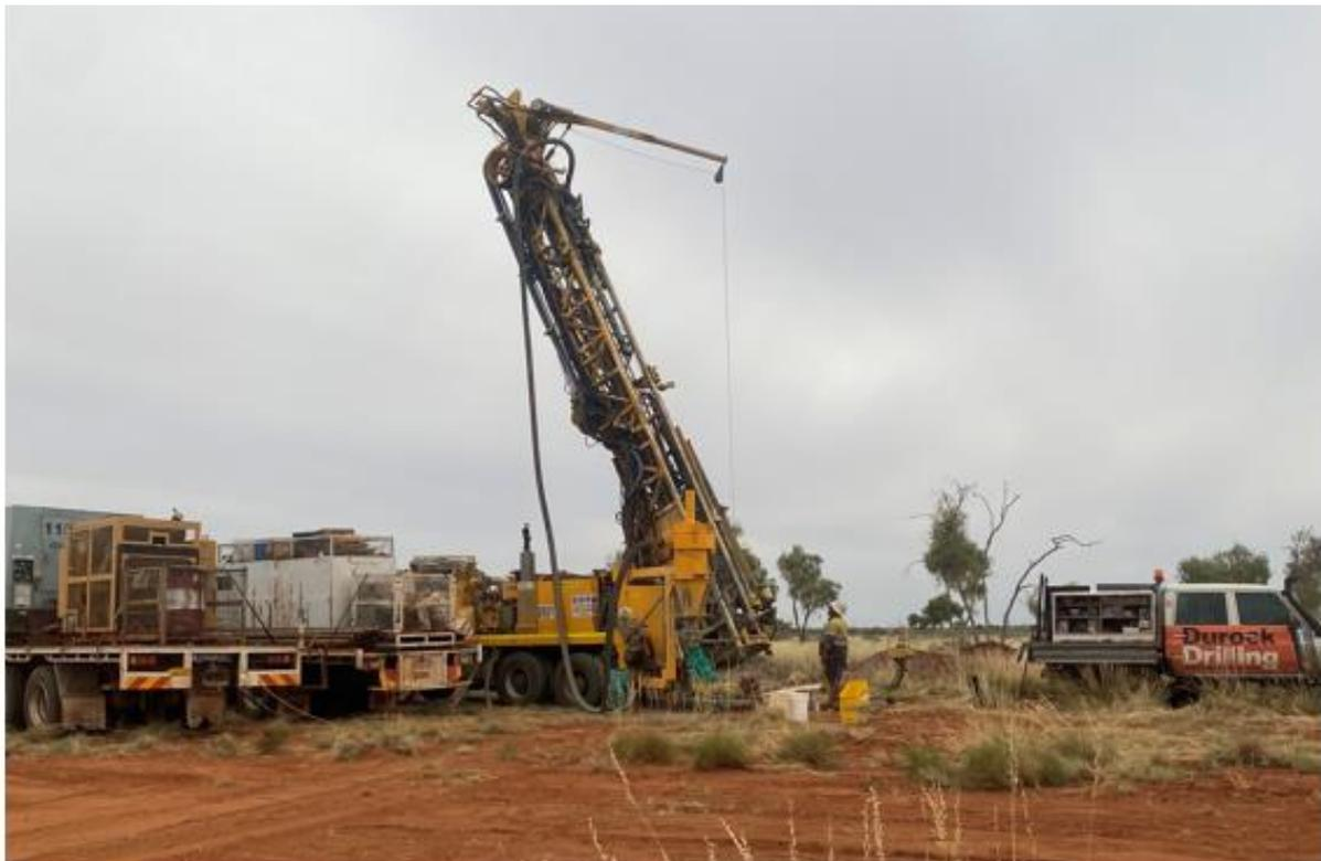
*Figure 4 – RC drill rig at Western Australian extension of the Arcee prospect*
