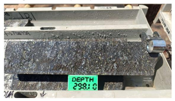
Figure 3. High grade copper mineralisation (as chalcopyrite) in Ore Schist unit from Nyungu Central (Hole NCDD004; core shown from downhole depth 298.1 metres)
