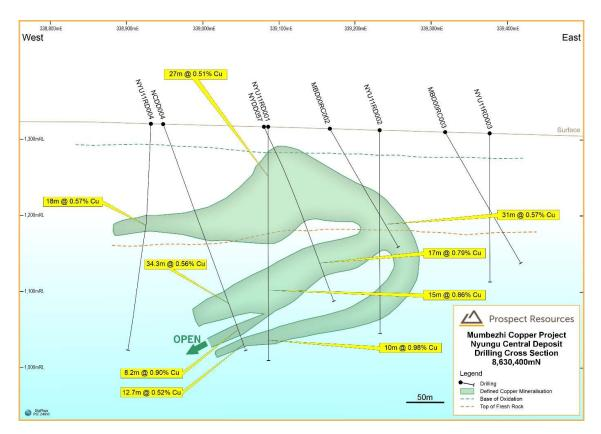
Figure 5. Drilling cross section at 8630400mN (showing NCDD004 intersection)
