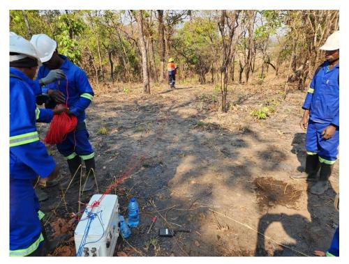
Figure 10: Geophysical IP surveying underway at the Kapikuba Prospect
