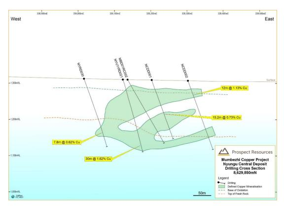
Figure 7. Drilling cross section at 8629850mN
