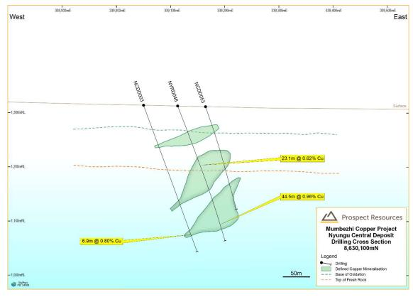
Figure 6. Drilling cross section at 8630100mN (showing NCDD003 intersection)
