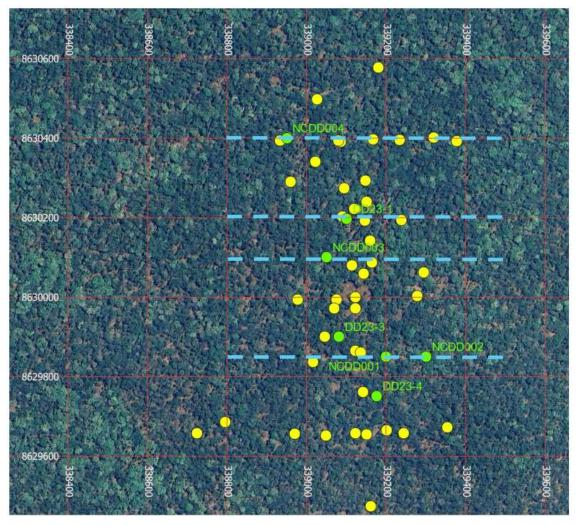
Figure 4. Nyungu Central drill hole collar plan showing sampled holes (green), historical holes (yellow) and drilling sections targeted to date (dashed blue lines)
