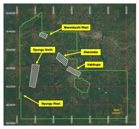
Figure 9: Mumbezhi exploration licence showing grid locations of IP surveys
