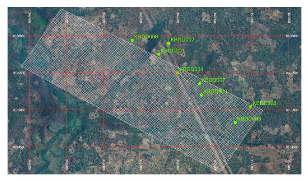
Figure 11: Geophysical IP survey grid over Kapikupa showing historical drill hole locations reported by Argonaut Resources NL in 2015
