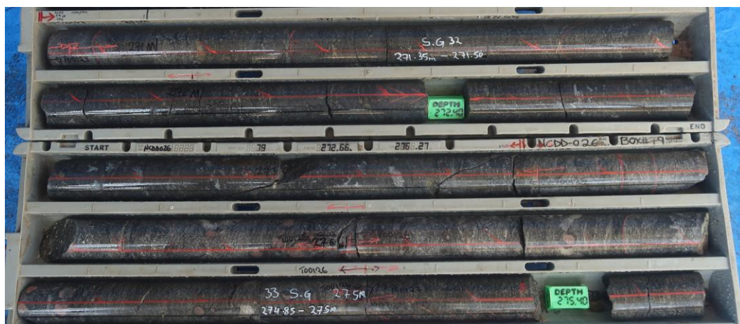
Figure 1. Diamond drill core photo of NCDD026 copper mineralisation 271.0-275.5m (est. grade 0.5% Cu)
