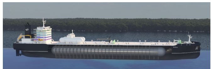
Figure 2: Illustration of Provaris' Proprietary Compressed H 2 Cargo Tank
