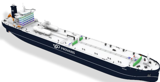
Figure 1: Illustration of the H2Neo 26,000m 3 compressed H 2 carrier
