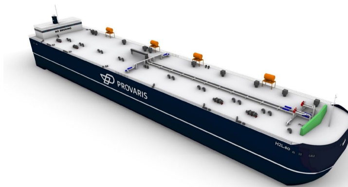
Figure 1: Illustration of the H2Leo 26,000m 3 compressed hydrogen floating storage
