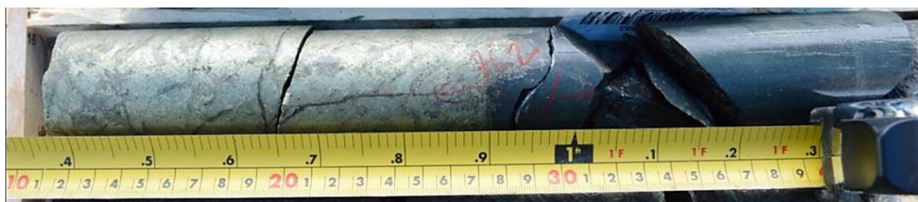
Figure 3: 0.25m massive chalcopyrite sulphide mineralisation, within 0.4m assaying 23.8% Cu, 0.1% Ni, 4 g/t Pd, 1.5 g/t Pt, 0.1 g/t Au from 75.8m (20-ZA-01). Forms part of wider 3.4m @ 5.1% Cu, 1.6% Ni, 2.1 g/t Pd, 1.1 g/t Pt. Drilled by Chase Mining in 2020.
