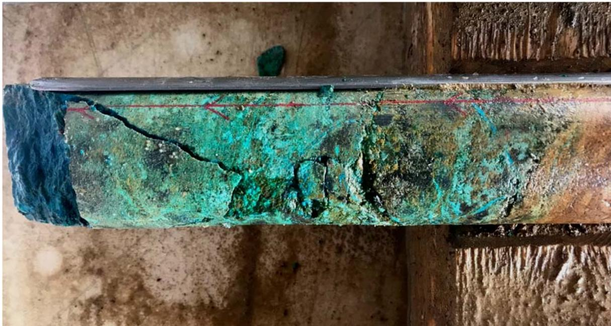
**Figure 5.** Intense copper oxide, mainly malachite in hole ZX-18020 pictured at a down-hole depth of 56.9m
