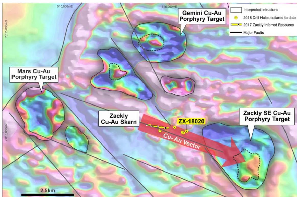
Figure 7. Aeromagnetic imagery showing a prominent magnetic anomaly to the SE of the Zackly inferred resource. Note the recently completed drill hole ZX-18020 in which thick zones of copper mineralisation were intersected, suggesting a possible vector of increasing widths of mineralisation towards the magnetic anomaly which represents a porphyry Cu-Au target
