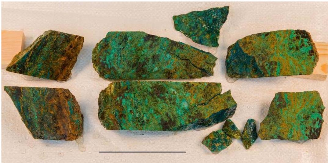
*Figure 1. Visible copper oxides in hole ZX-18020, 56.67 to 57.00m down-hole depth (scale bar = 10cm)*
