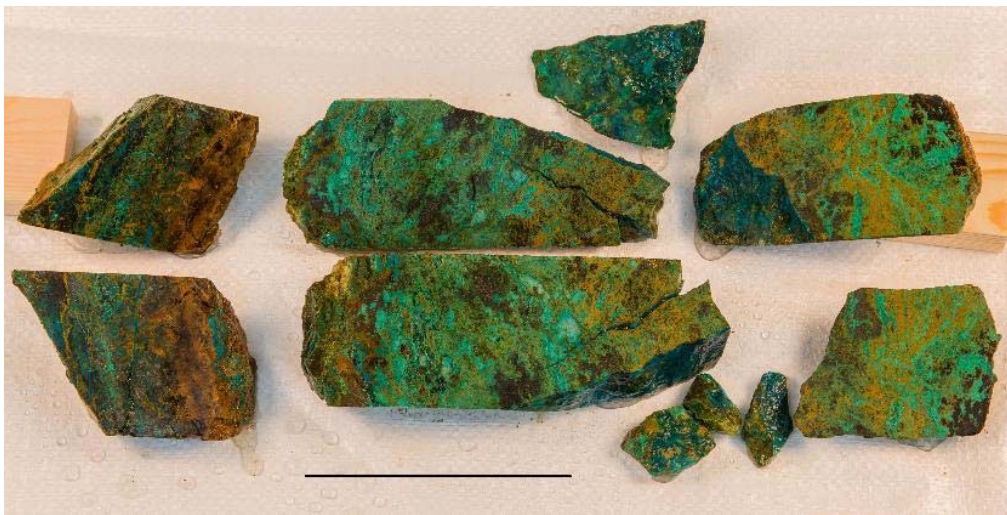
Figure 1. Visible copper oxides in hole ZX-18020, 56.67 to 57.00m down-hole depth (scale bar = 10cm)
