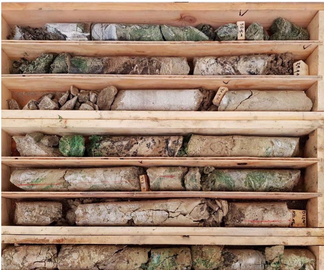
Figure 6. Visible copper oxide mineralisation in drill hole ZX-18020 in strong garnet skarn alteration nearer surface.
