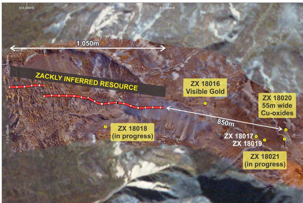
Figure 4. Drill hole plan for Zackly showing the 2017 surface trace of PolarX's inferred resource outline (red) and the initial 2018 drill holes collared to date (yellow) on detailed drone imagery.
