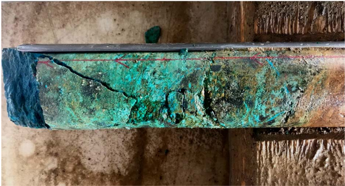
Figure 5. Intense copper oxide, mainly malachite in hole ZX-18020 pictured at a down-hole depth of 56.9m
