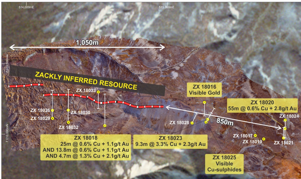
Figure 2. Drill hole plan for Zackly showing the 2017 surface trace of PolarX's inferred resource outline (red) and the 2018 drill holes collared to date (yellow) on detailed drone imagery.
