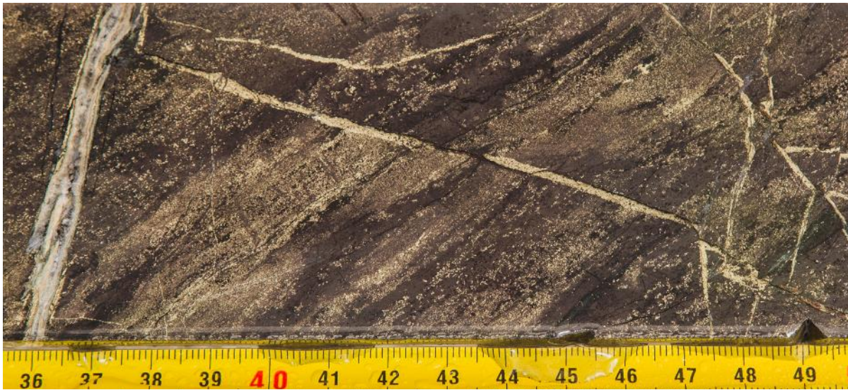
Figure 4. Visible copper sulphides and magnetite in half-core, hole ZX-18025, 93.8m down-hole depth. Copper sulphides comprise mainly chalcopyrite (yellow colour). Note multiple generations of mineralisation, with earlier disseminated chalcopyrite replacing relict bedding and subsequently overprinted by fracture hosted chalcopyrite. Scale bar is in cm.
