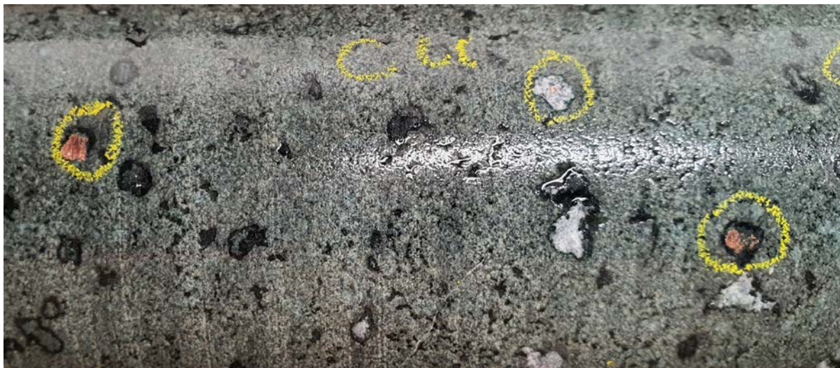
Figure 3 Native copper mineralisation in vesicle infill within porphyritic andesitic-basalt lava flows, 21.35m depth in drill hole CD21-008. Core is approximately 6cm in diameter.
